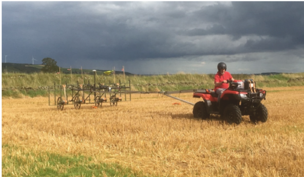
Multi-sensor gradiometer array in Area 1
