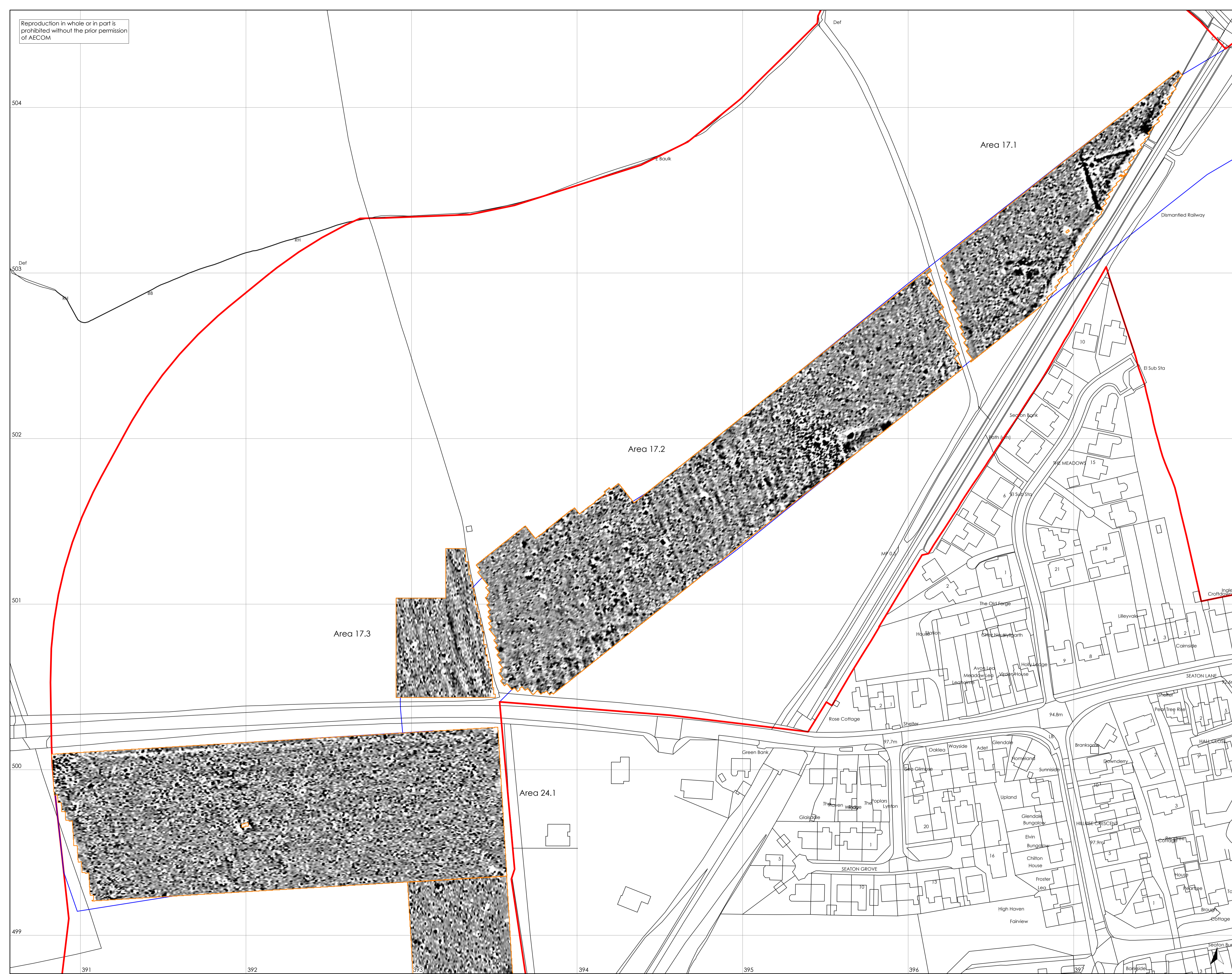
Figure 10: Areas 17.1-3 & 24.1 - Magnetometer survey
