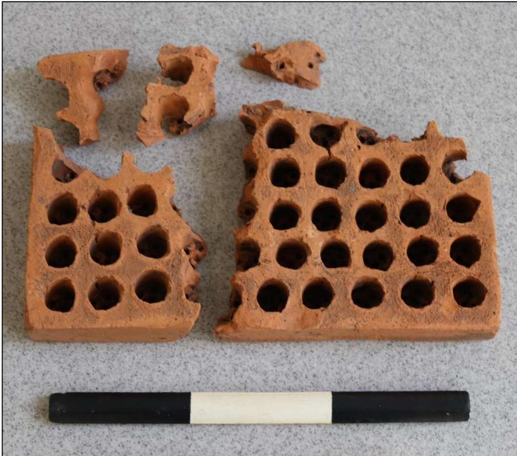
Photograph 99 (above): The underside of one of the maltkiln tiles. The holes stop short of the upper surface
