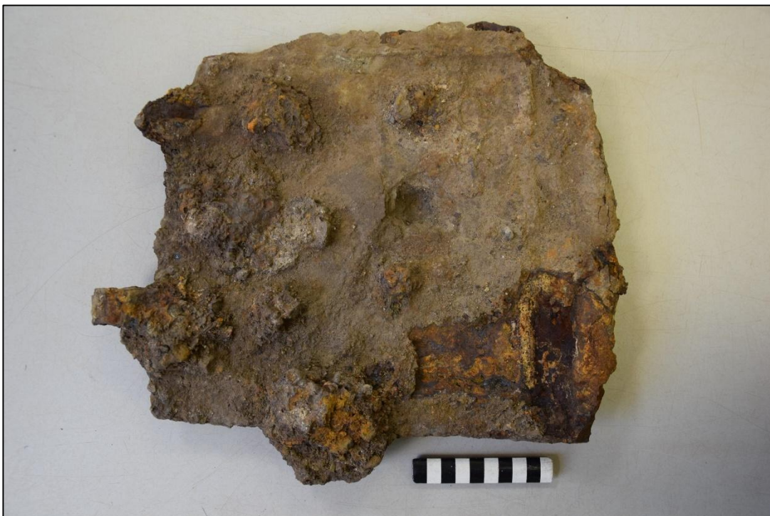
Photograph 84: The iron door from the small hearth at the Newcastle kiln, with the hinges at the left and a flange to cover the junction with a matching door at the right. A block of rust has fallen off to reveal the moulded frame, lower right
