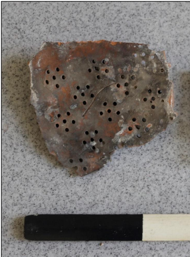
Photograph 99 (above): The underside of one of the maltkiln tiles. The holes stop short of the upper surface
