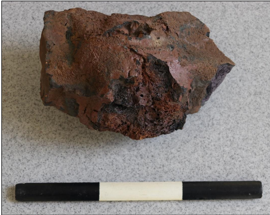
Photograph 95: Another example of failed firing; the brick is distorted and broken
