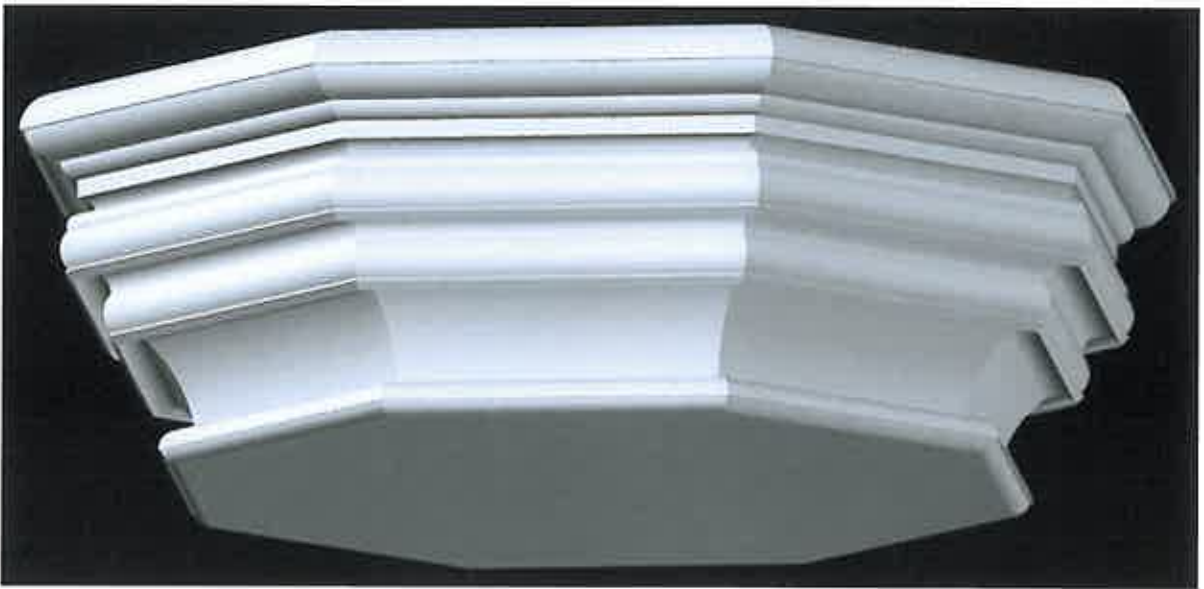
Figure 8. Goodrich Castle. Final design Solar Arch Pier Capital
