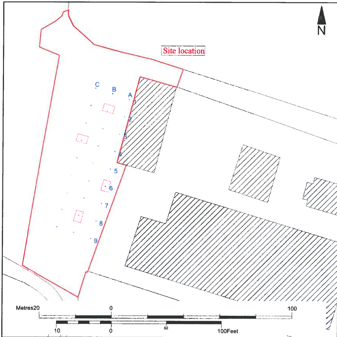
Plan showing the outline of the building and the bore hole sampling grid.
