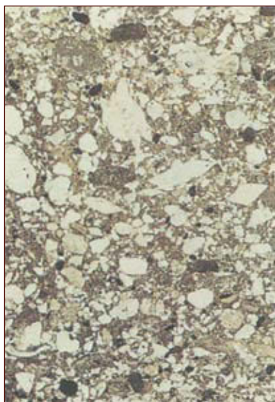
[69] Medium plaster Type 106. Side of southern altar. Thin-section 93.4, Unit 7. Plane polarised light. Frame height: 7.2 mm.
