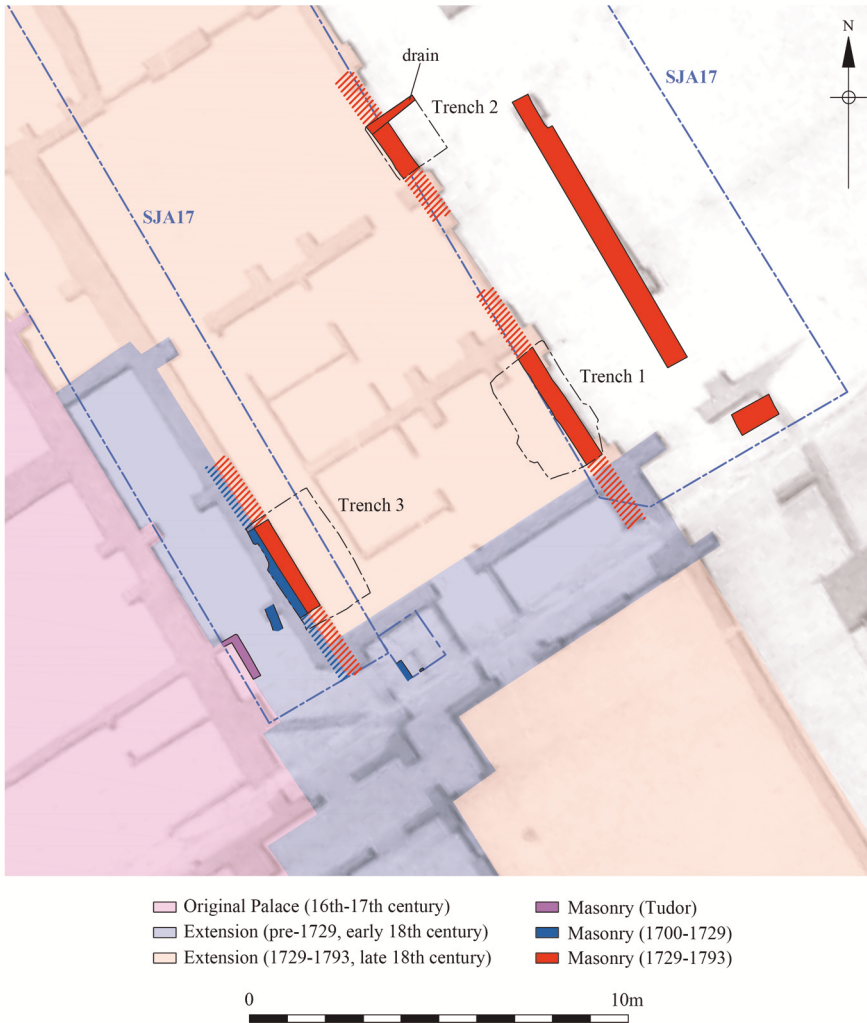
Fig 4: 16th- and 18th-century masonry overlaid on to the 1793 Floor Plan
