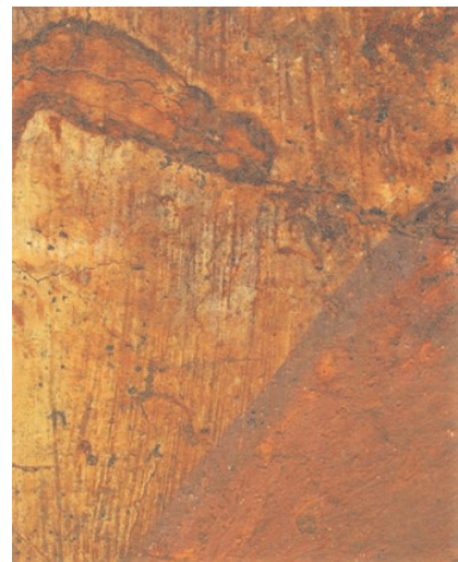
Fig 15: another fragment of wall plaster that clearly shows the vertical brush strokes
