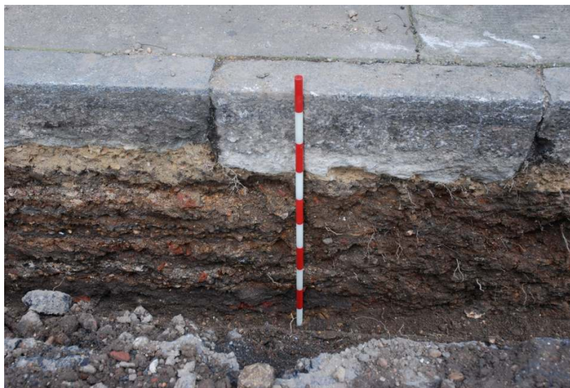
Figure 17: South facing section of trenching on Nelson Place showing mixed made-ground and rubble layers (1m scale).
