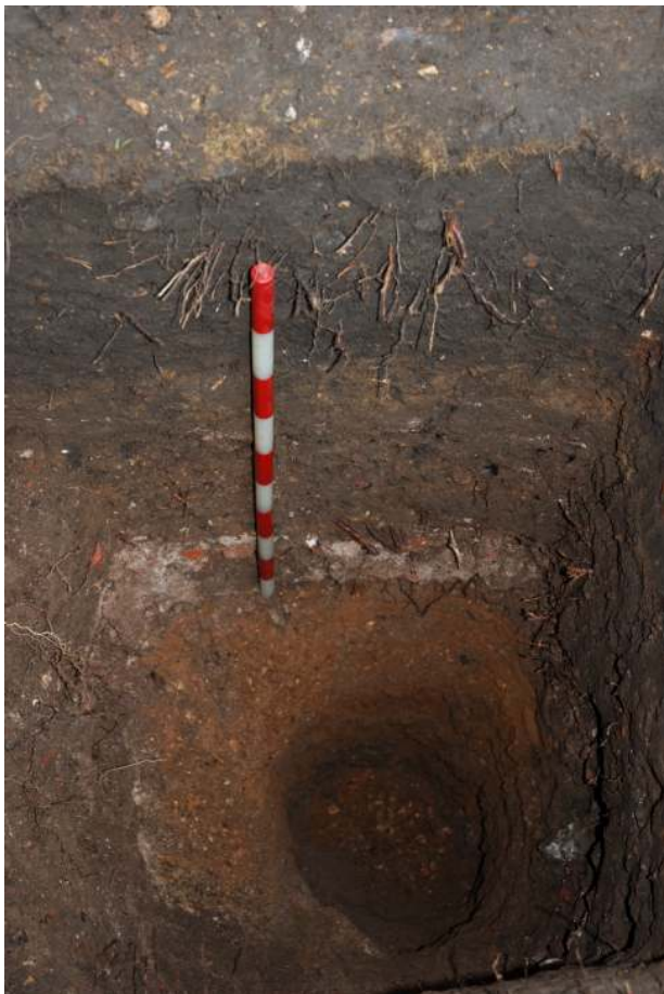
Fig. 53: Photo of trial pit 15, with the brick rubble layer and 'natural' deposit clearly visible towards and at the base of the scale.
