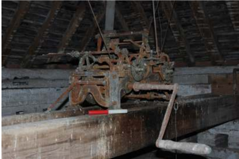
Fig. 134: Photograph of the clock, showing the winding handle attached to the striking train.
