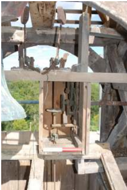
Fig. 144: Photograph of the bell and upper clock mechanism or motion-work, contained in a small wooden casing behind the clock-face.
