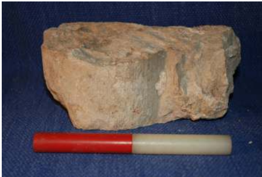
Fig.19: Reigate moulded stone re-used in Aldgate wall, (0.2m scale)
