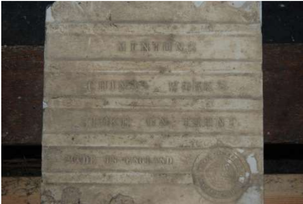
Fig. 240: Close-up of the rear of a Minton tile, with the 'Made in England' stamp.
