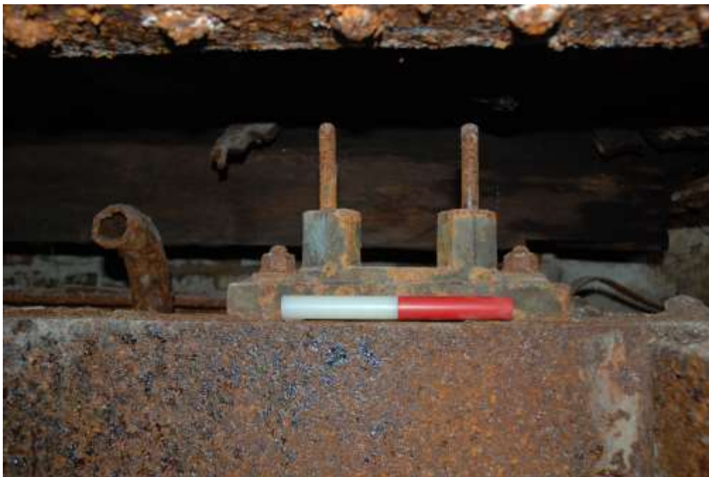
Fig. 111: Photograph of the support bracket, which would have held the bell-cranks which turned the actuating rods on a 90° angle.
