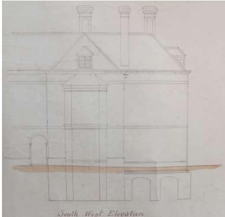
Fig. 172: 1899 southern elevation, depicting a deep solid wall below ground level probably for a cellar.
