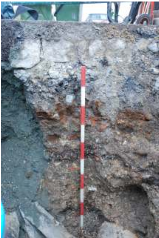
Fig. 30: Photograph of one of the pits on Eagle Wharf Road, showing the disturbed service backfills (left side of image) and layers of made-ground deposits (right side of image).
