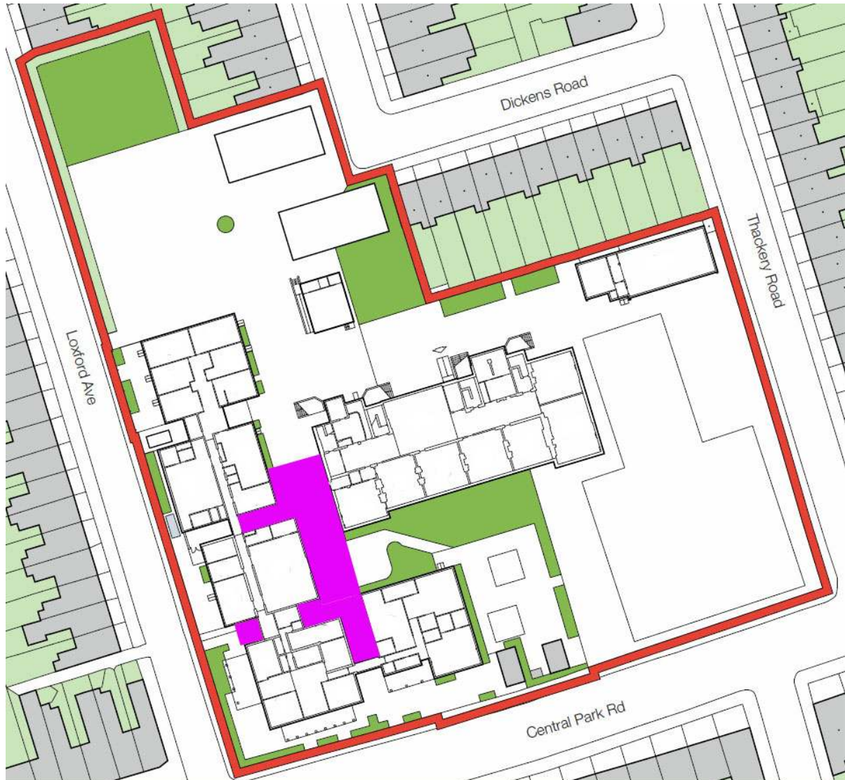
Fig.32: Ground-floor plan of the site, showing the areas of the proposed extension (in pink)
