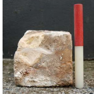
Fig.40: Block E showing notch and tool marks, (20cm and 50cm scales)
