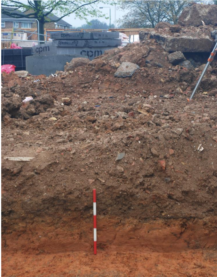
Fig. 24: Exposed section midway along the northern side of Area 4, showing c 200mm of made ground over the natural deposit (0.5m scale)
