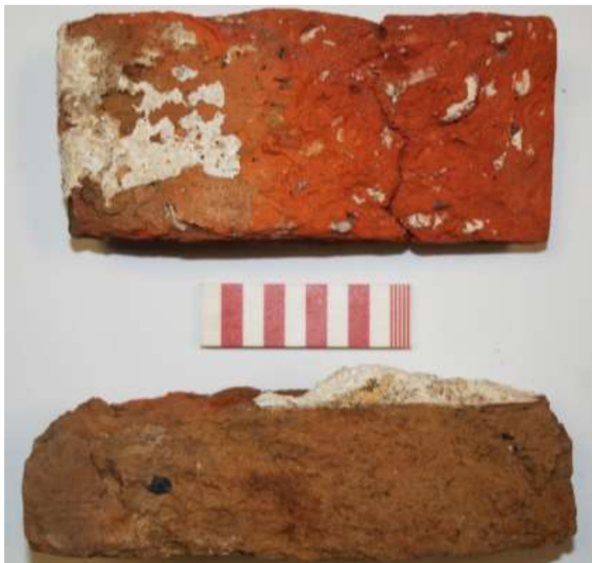
Fig.69: Sample bricks from the main body of the east-west retaining wall (7). 100mm scale
