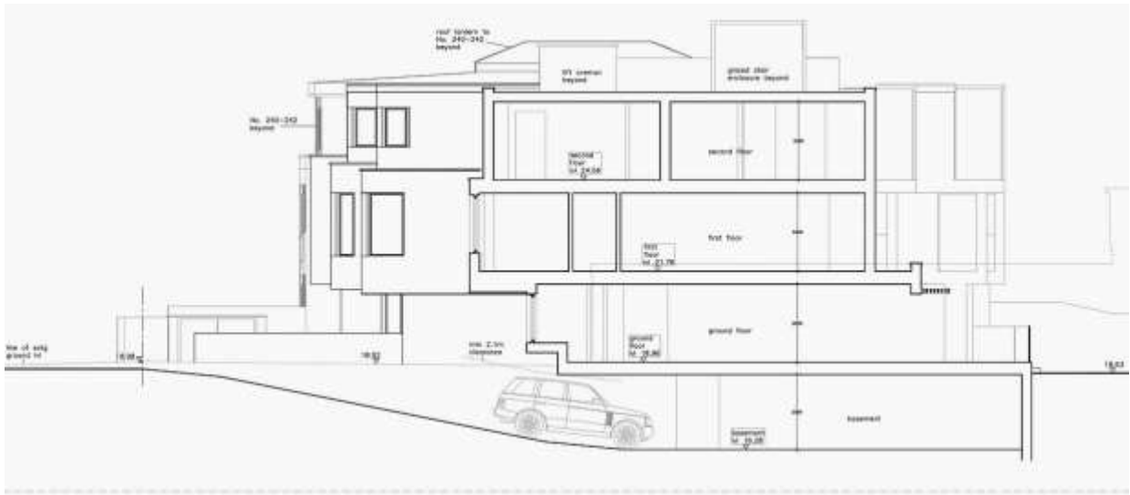
Fig. 3: Proposed section N-S. (Extracted from drawing no. 1182/08 revision A by Form Architecture).
