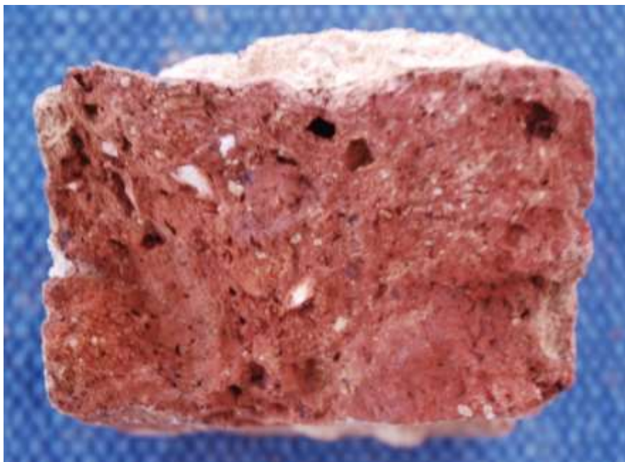
Figure 30: Cross-section of 18 th /19 th century brick from [9]
