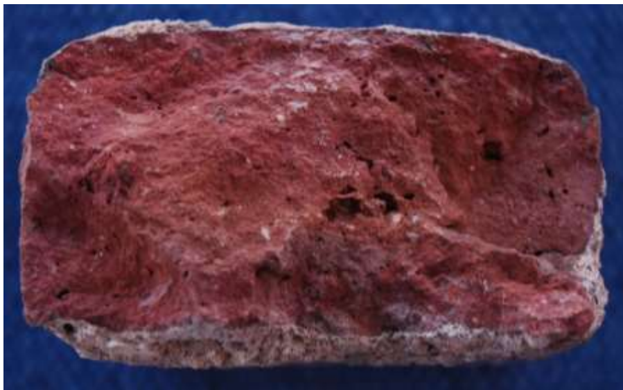
Figure 32: Cross-section of 17 th century brick with 'cleaner' fabric from [9]
