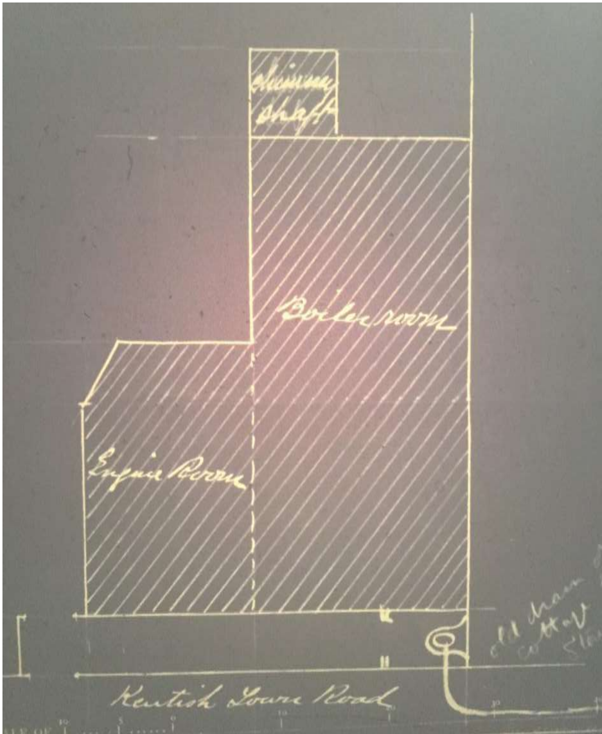
Figure 31: Plan of the steam pumping house. Regent's Canal on the left. (Taken from planning application, 1926)
