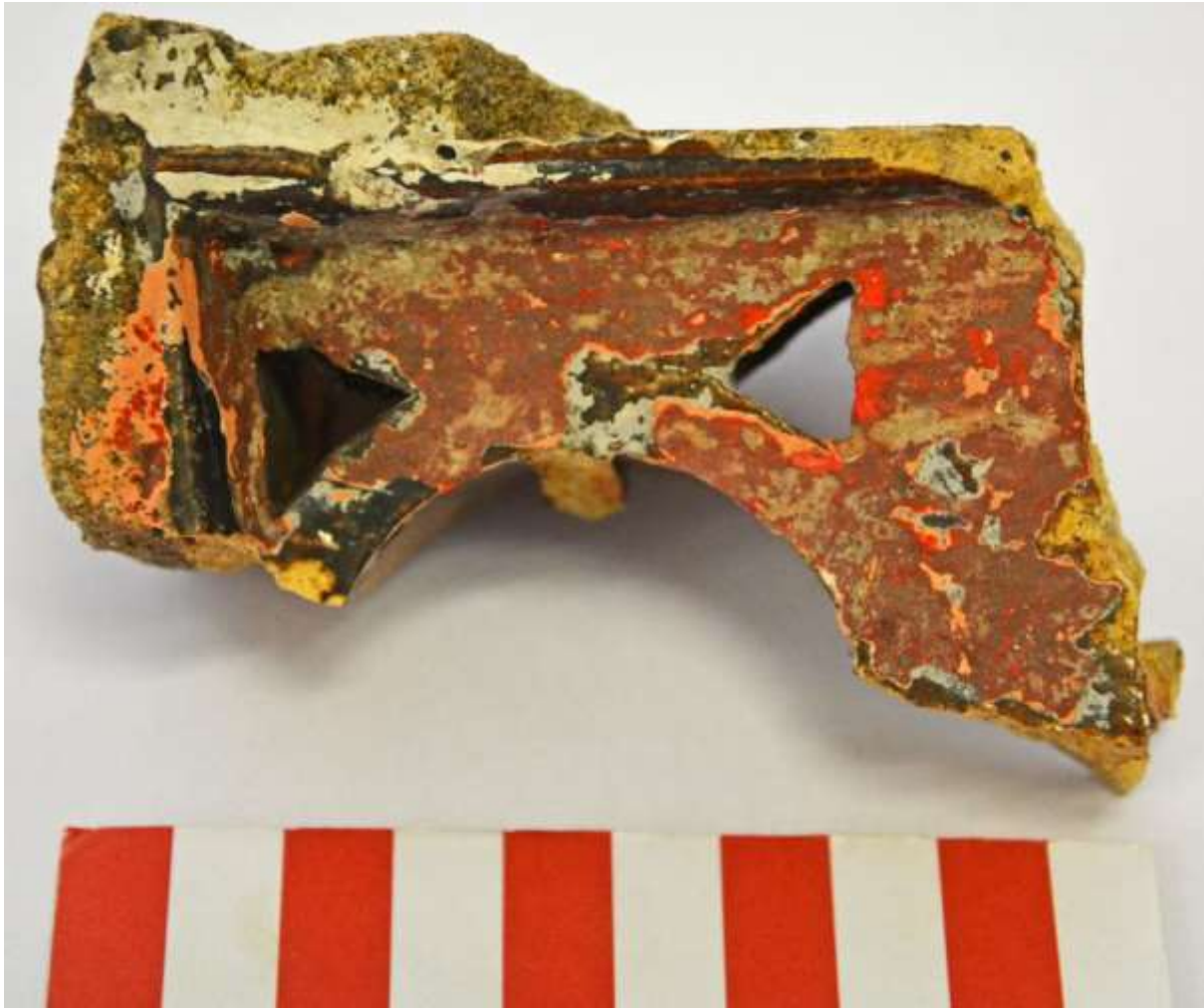
Figure 83: Fragment of ceramic ventilator showing layers of paint over the original brown glaze. Scale 0.1m
