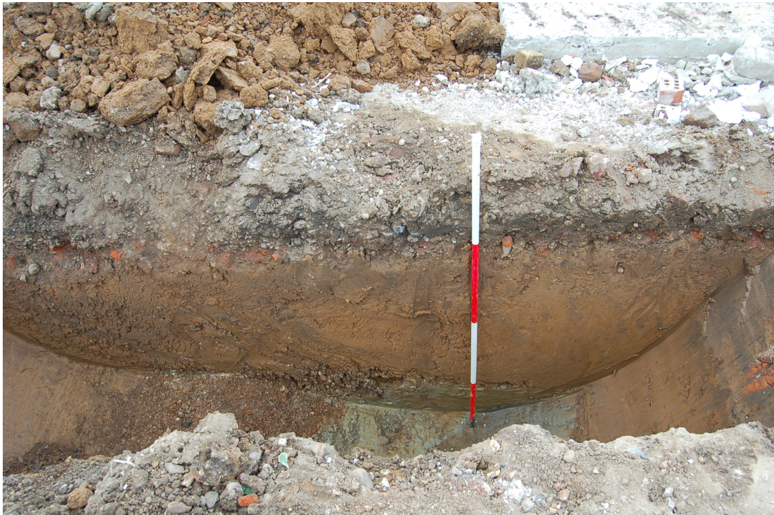
Fig 9 View of Trench 3 looking towards the northwestern section (2m Scale). The depths of concrete and firm alluvial clay can be clearly seen. The gravel is just evident above the last red block of the scale and the stiff blue/grey clay can be seen appearing below this point and does continue under the gravel to the left of this image.
