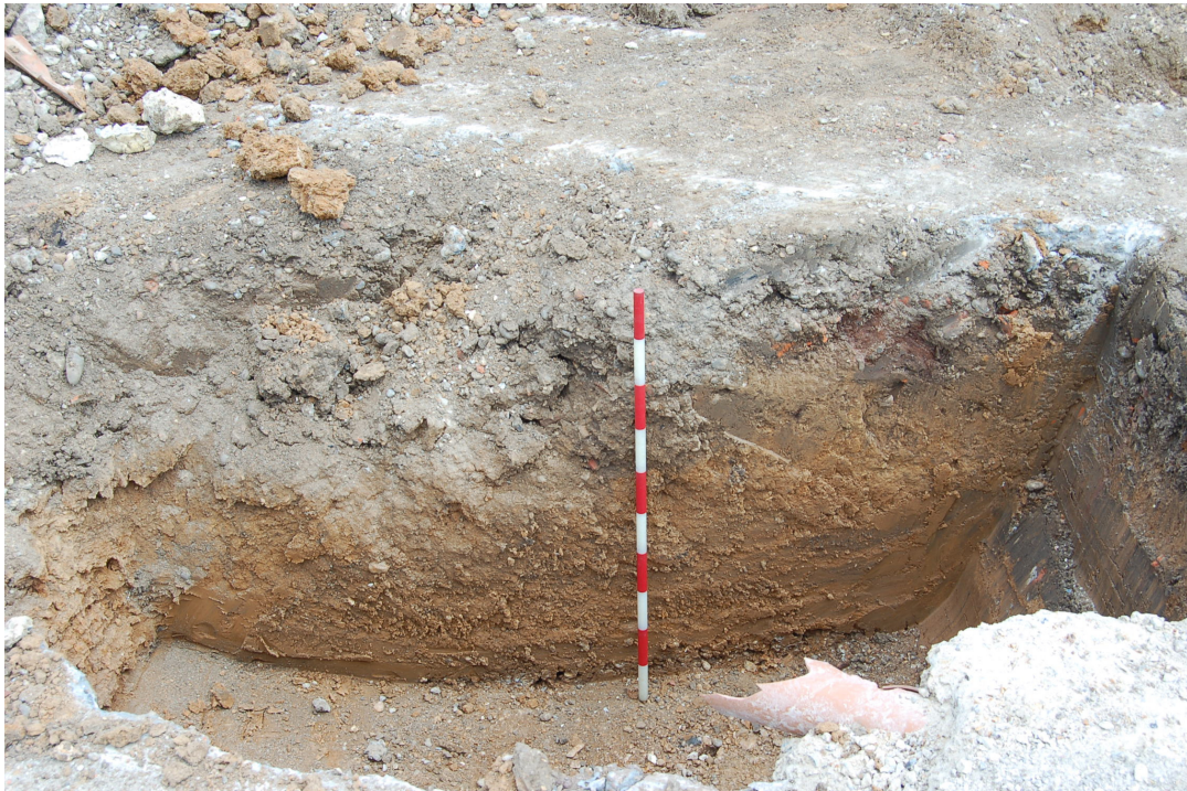
Fig 7 View of Trench 1 looking towards the northwestern section (1m scale). The depths of concrete and firm alluvial clay can be clearly seen. The gravel is just evident at the base of the trench.
