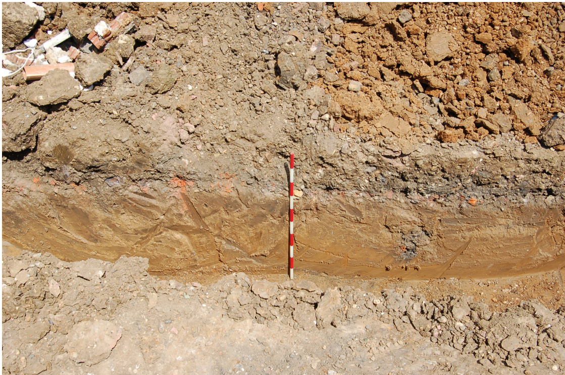
Fig 10 View of Trench 4 looking towards the northeastern section (2m Scale). The depths of concrete and firm alluvial clay can be clearly seen. The gravel is just evident at the base of the trench.
