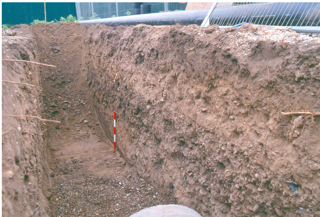
Fig 19 Drawn section through the buried stream channel [7] and overlying deposits (located on Figure 15). Below - views on the southern side of this feature looking north and east, with the waterlaid silt deposit [6] visible at base (0.5m scale)
