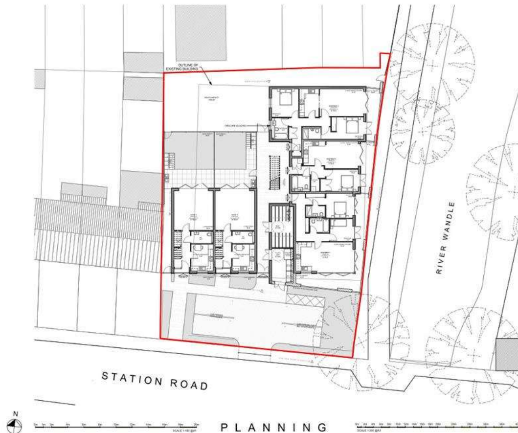
Figure 6: Proposed ground floor plan of new development, with site outline marked in red. Adapted from drawing 001/PL/201 supplied by the Client.
