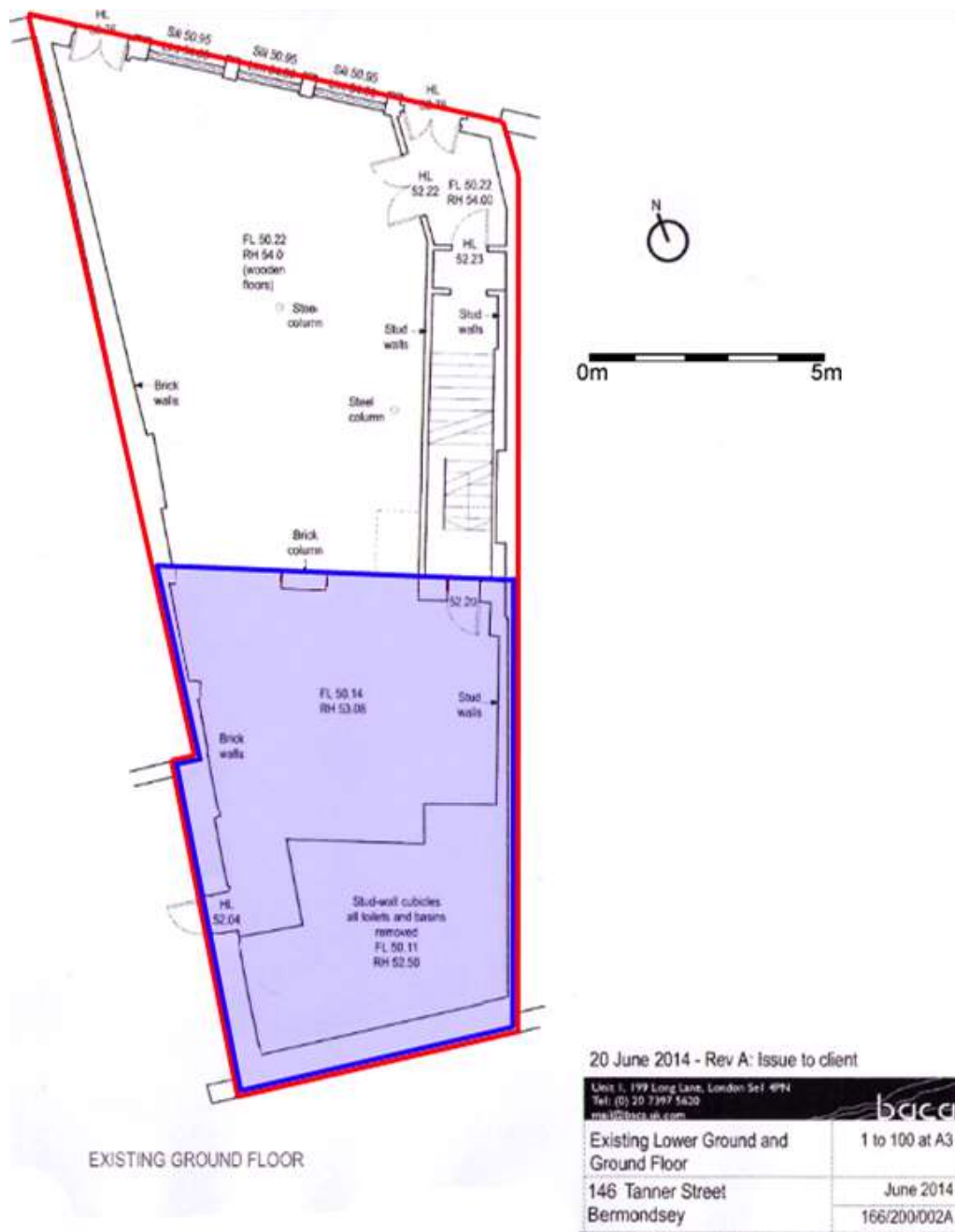
Fig. 7: Plan of the existing site showing property boundaries (red) and works area (blue); based on a plan by Anderson Consulting Engineers & supplied by the Client.
