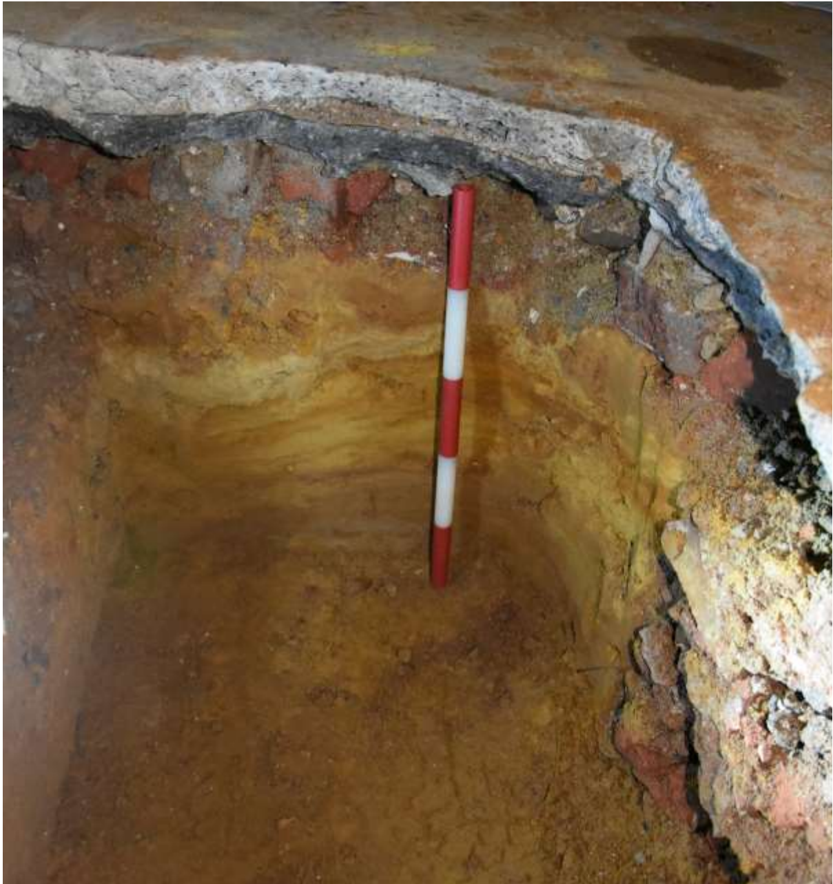
Fig.13: Test pit 7, facing ESE, 0.5m scale. Note the layers of compacted sand forming natural geology immediately below the previous slab formation level.
