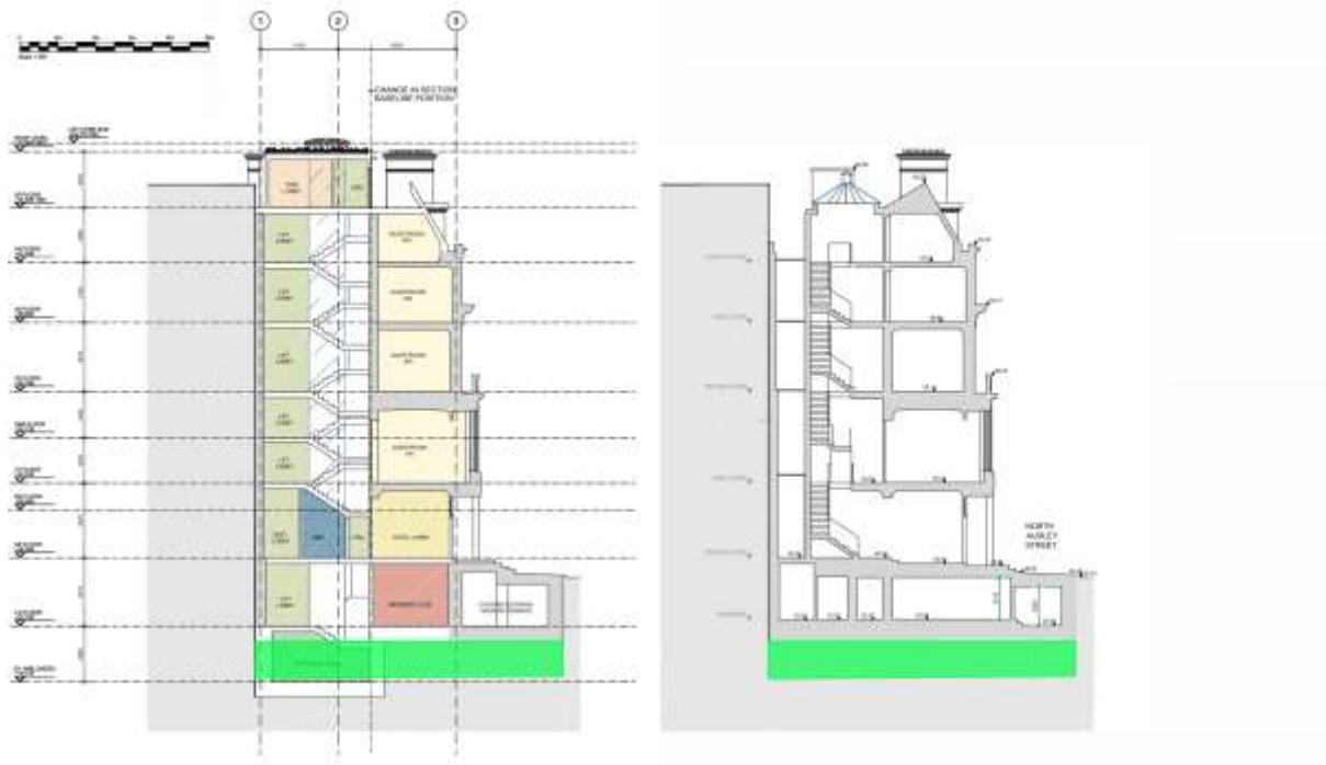
Fig.35: Section through proposed and existing site with indication of depths of made ground. West to the left and east to the right on each drawing
