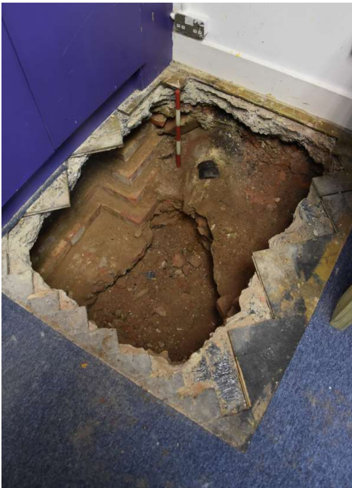
Fig.16: Test pit 3 facing NW, 0.50m scale. Note the surrounding footings, concreted pipe, and the associated made ground
