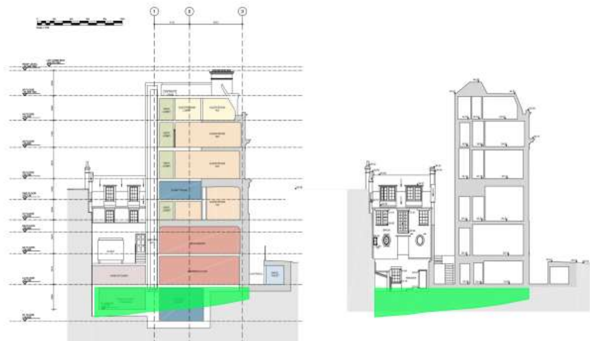
Fig.36: Section through proposed and existing site with indication of the depth of made ground. West to the left and east to the right. Lees Place to the left, 22 Grosvenor Square and 43 North Audley Street to the right.
