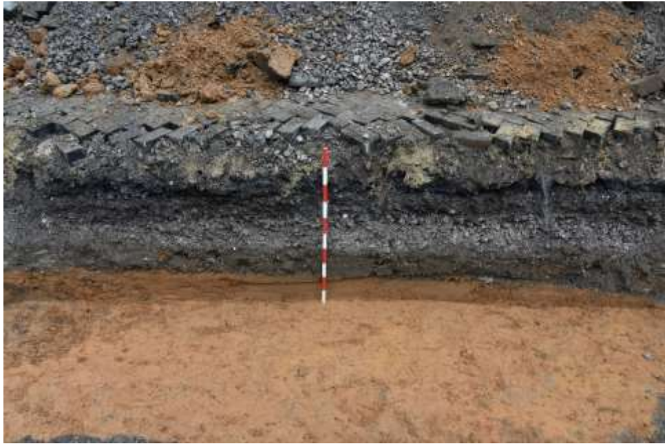
Fig 12: NW facing section, Trench 1, highlighting the Made-ground layers (1m scale).
