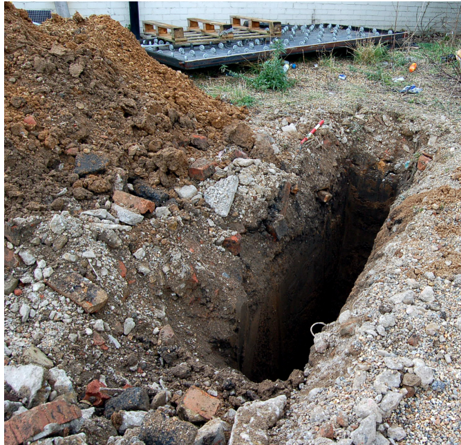
Fig. 8 The north facing section of test pit 7, please note that for health and safety access reasons the test pit could not be examined from within the trench (scale: 0.5m)
