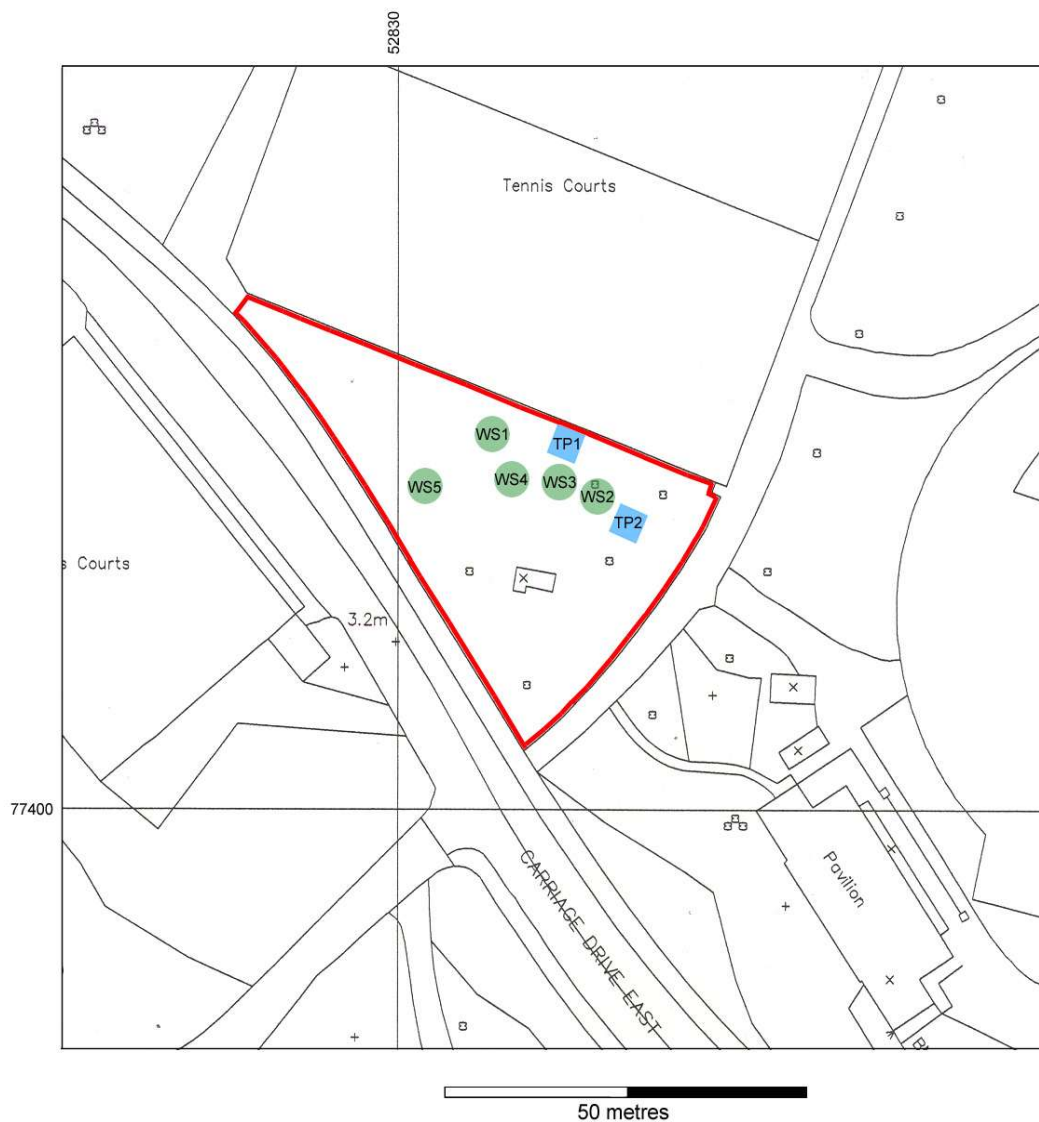
Figure 3 Site plan showing the approximate location of the two test pits (blue) and the five window samples (green). The size of the TPs and WSs is obviously shown at a larger scale for identification purposes.
