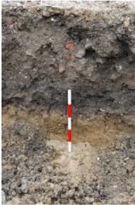
Figure 10 The section of trench 2, showing the made ground deposits over natural sands
