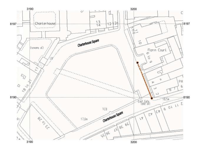
CQE04: Line of the service trench excavation (highlighted) in relation to the current Ordnance Survey map. Scale 1:1000
