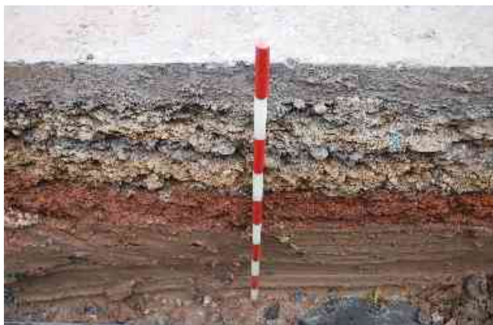
Fig 12: The west facing section of a feeder trench at the eastern end of Ladbroke Square with clearly defined stratigraphy ( 1m scale ). A series of road make up deposits overlie the truncated surface of natural London Clay, which is at its highest only 380mm below the current road surface, therefore visible at a height of circa +26.2m OD.
