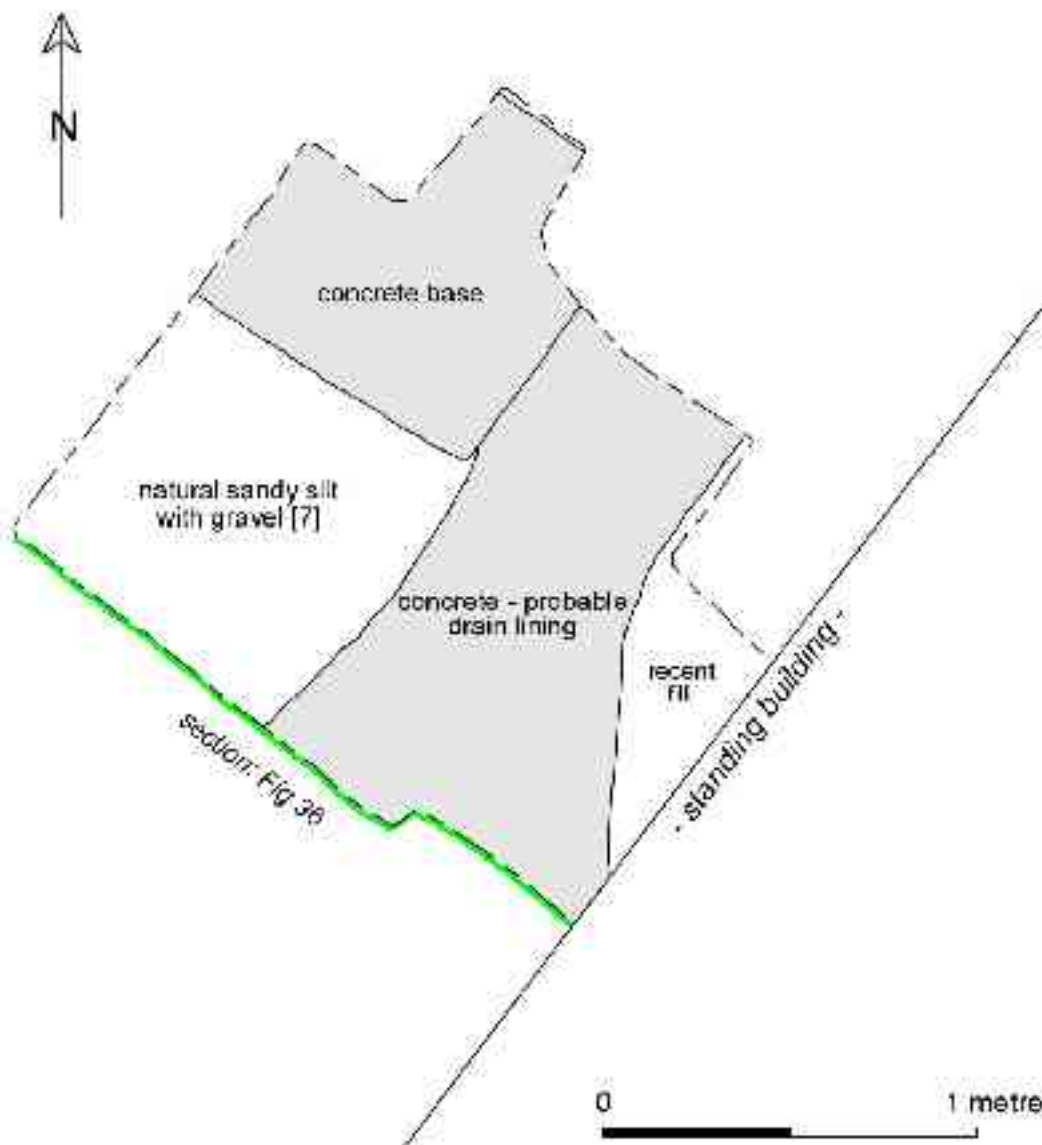
Fig 34 Plan of Test Pit 3, showing the substantial obstruction caused by in situ concrete features
