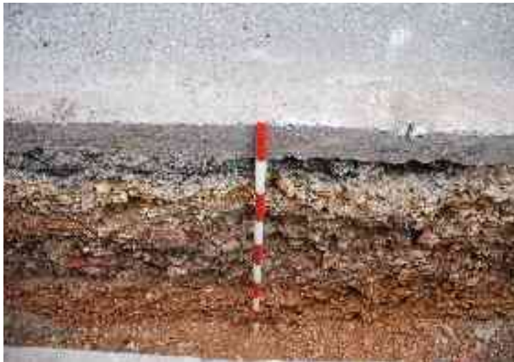
Fig 12 (left) east-facing section of an open cut trench on Albion Street showing the rubble-based made ground below the road make up layers and the natural terrace gravel at the base of the trench.
