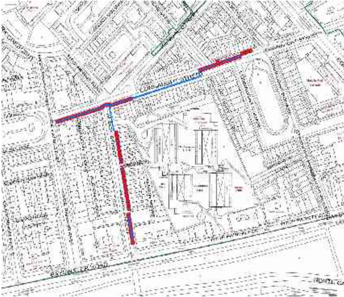
Fig 7 The Victorian Mains Replacement works in Barrow Hill District Metering Area 30, showing the line of the VMR works in blue (insertion, open cut and drilling). The open-cut trenches and pits that were monitored during the watching brief are highlighted in red.
