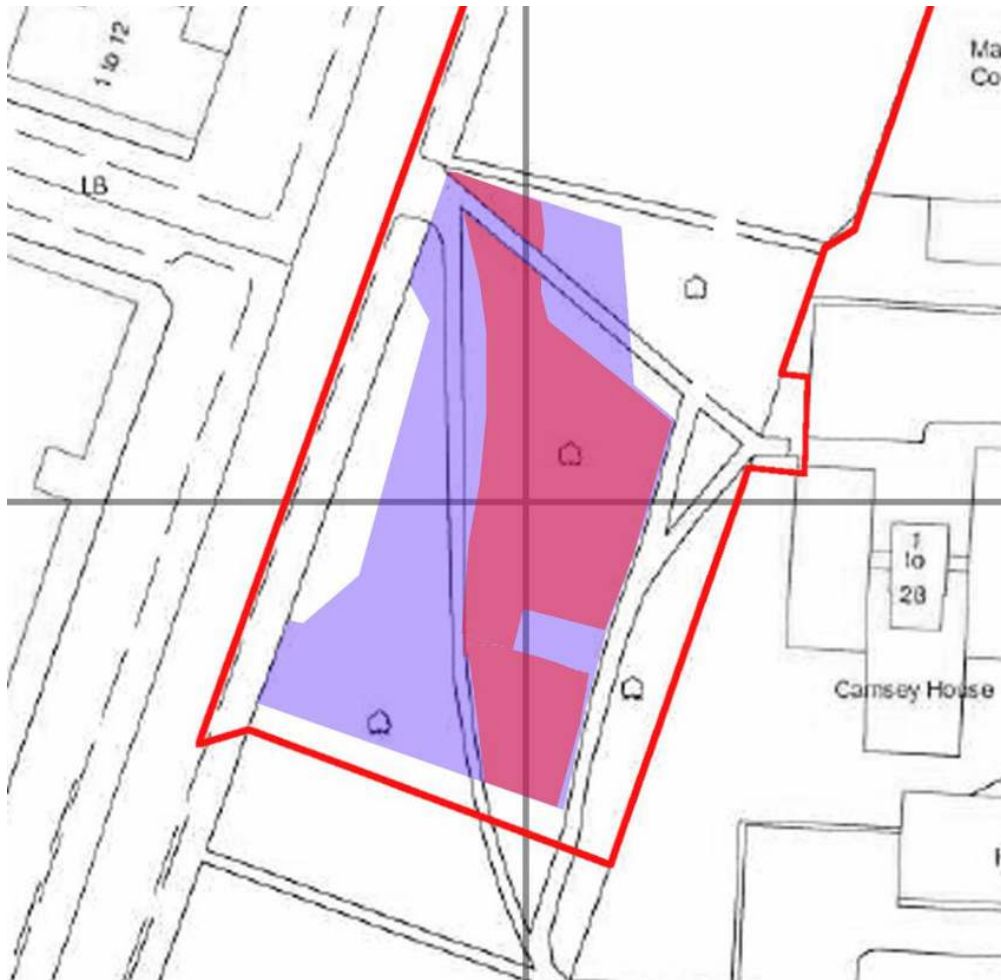
Figure 12: Machine stripping in Area B (red) and the perimeter of the site compound (blue).
