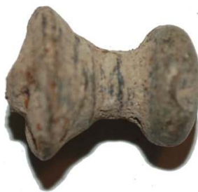
Figure 21: SF23, Copper alloy bureau knob, up to 12.5mm diam. x 14mm long.
