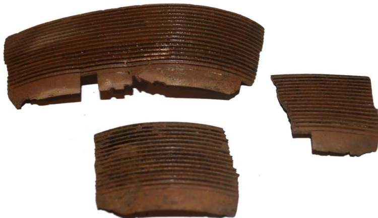
Figure 39: SF2-4, shrapnel fragments. The pieces are 21.5mm wide by \leq 1.8 mm thick; one 67mm long and the other two fitting together to form a strip 54mm long.
