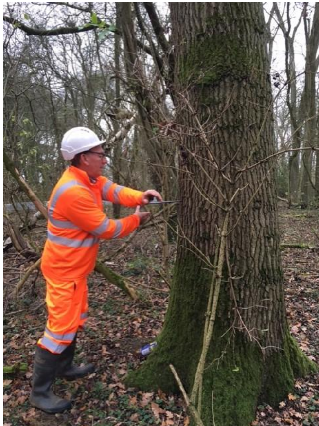
Figure 3a/b: Haglof Corer (top), with coring in progress (bottom)
