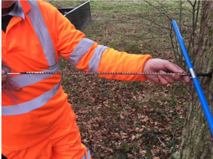
Figure 3c: Extraction of core sample from the corer
