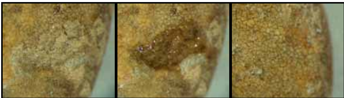
Figure 4. The process of cleaning with rewetting the accretion. Left: the accretion, Middle: the accretion wetted, Right: the accretion removed. (No. 200434974)
