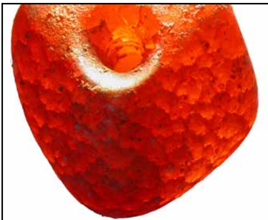
Figure 2. The cracks in amber become visible when light penetrates the bead (No. 200434975)
