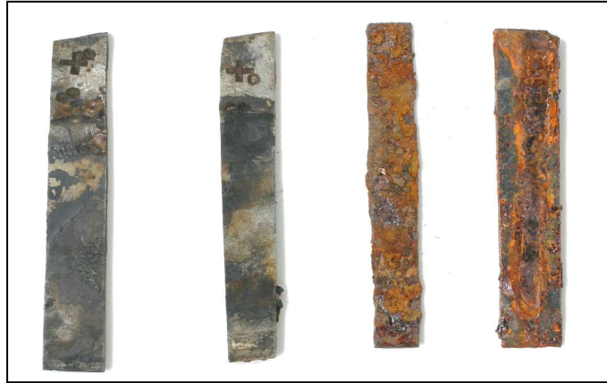
Figure 6. Comparison of coupons 2, 4, 6 and 8 (left to right) from Cluster 2, Rod 2, after 6 months' burial. Coupons 2 and 4 exhibit thin dark corrosion products indicative of reduced species, whereas coupons 6 and 8 reveal orange and brown corrosion products indicative of oxidised species.
