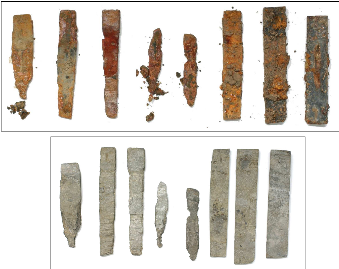
Figure 5. Iron samples from Cluster 1, Rod 4, after 30 months' burial. The upper photograph shows coupons 1–8 (left to right) as recovered and after removal from the installation rod. The lower image shows the same coupons after chemical stripping.
