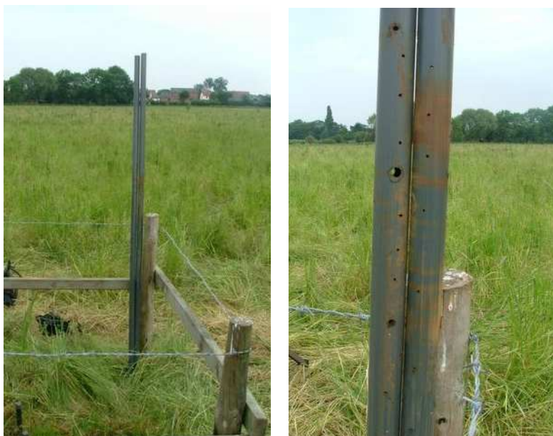
Figure 10. Iron staining visible as rings around the tubing used for the bone burial experiments removed from Cluster 2 at 30 months. When in the ground, the tubes are proud of the soil surface by c. 0.2m which means that the widest iron staining ring (visible at the top of the right image) is c. 0.5m below ground level, and the lesser iron staining rings (visible below the widest ring) are deeper in the ground. Photos: Matthew Collins
