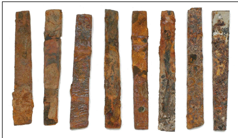
Figure 4. Iron samples from Cluster 1, Rod 3, after 18 months' burial showing coupons 1–8 in sequence, with coupon 1 at the left. Coupons 1 and 2 show typical orange-red accretions over black deposits, whereas coupon 3 reveals a lustrous layer of relatively thin corrosion products. Coupons 4 to 7 show both orange and black corrosion products. Coupon 8 (right) has some bare metal (visible at the top) plus a thin layer of orange and brown corrosion products.
