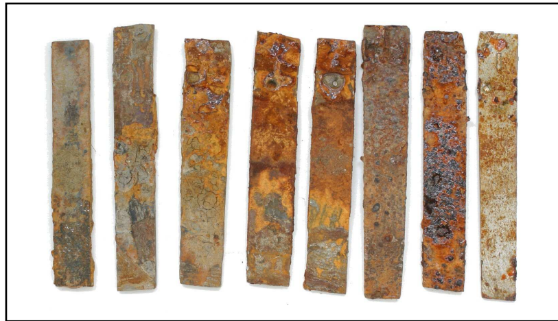
Figure 3. Iron samples from Cluster 1, Rod 1, after 6 months' burial showing coupons 1–8 in sequence, with coupon 1 at the left. Note that the coupons at either end are less corroded than those in the centre. Coupon lengths, c.50mm.
