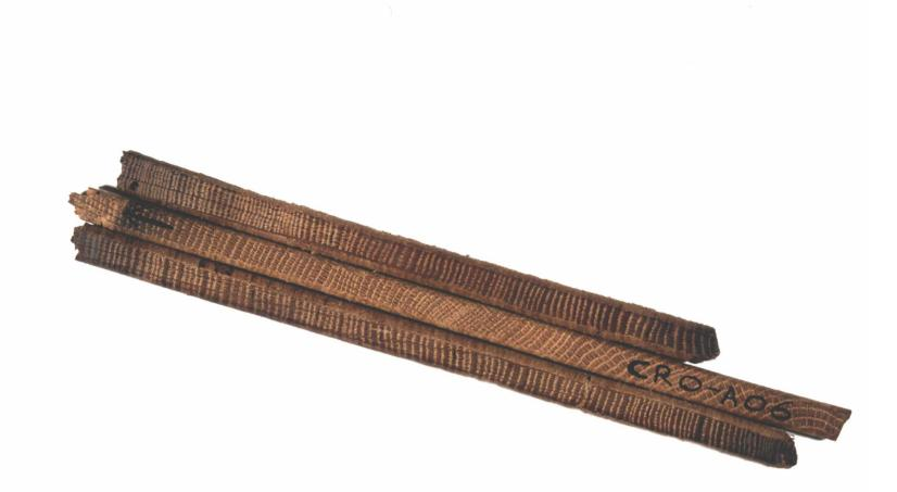
**Figure 4:** Three cores from timbers in a building. They come from trees growing at the same time. Notice that, although the sequences of widths look similar, they are not identical. This is typical.
