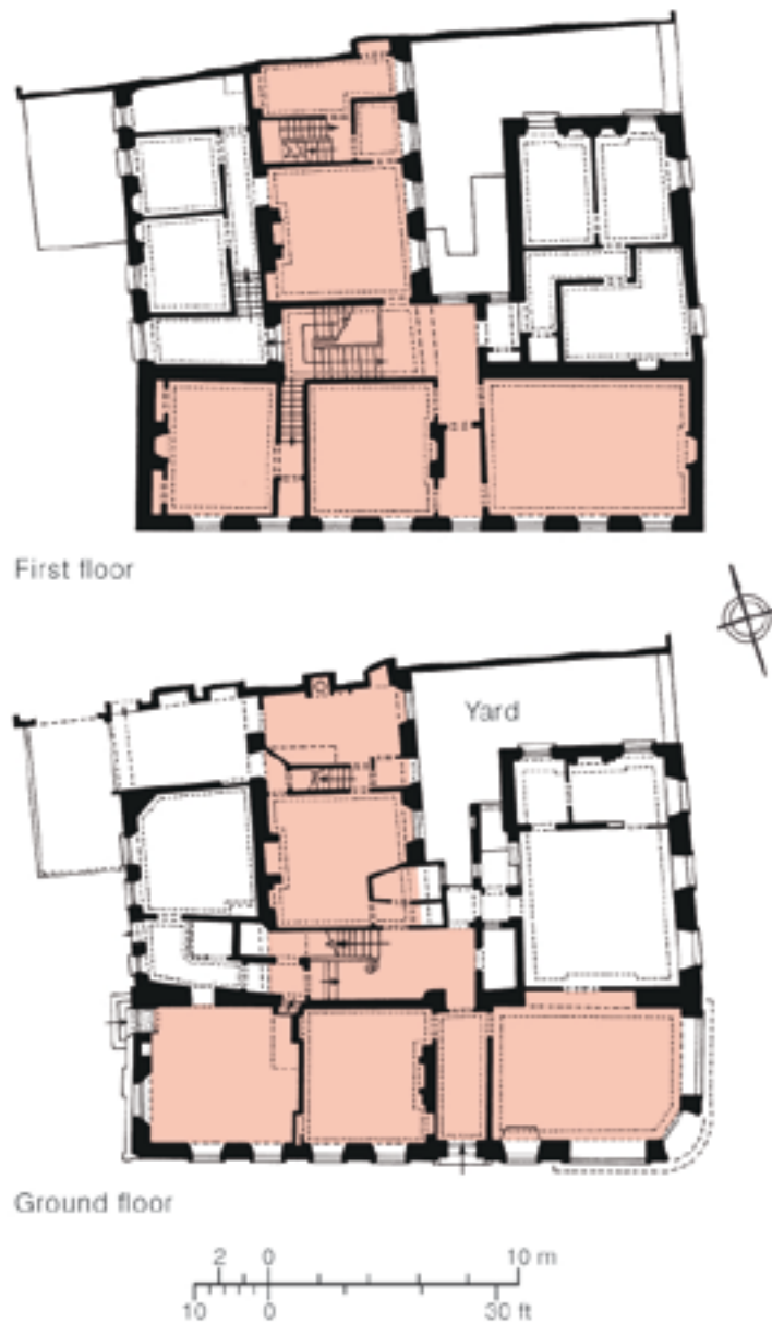
Fig. 12: Plans of the ground and first floor of 2 Love Lane / 64 West Street. The principal mid-18th-century building phase is shaded pink. The original form of the stair compartment's eastern end is uncertain. The south wall of the granary (60 West Street) forms the northern boundary of the yard and the wing of the house. © English Heritage
