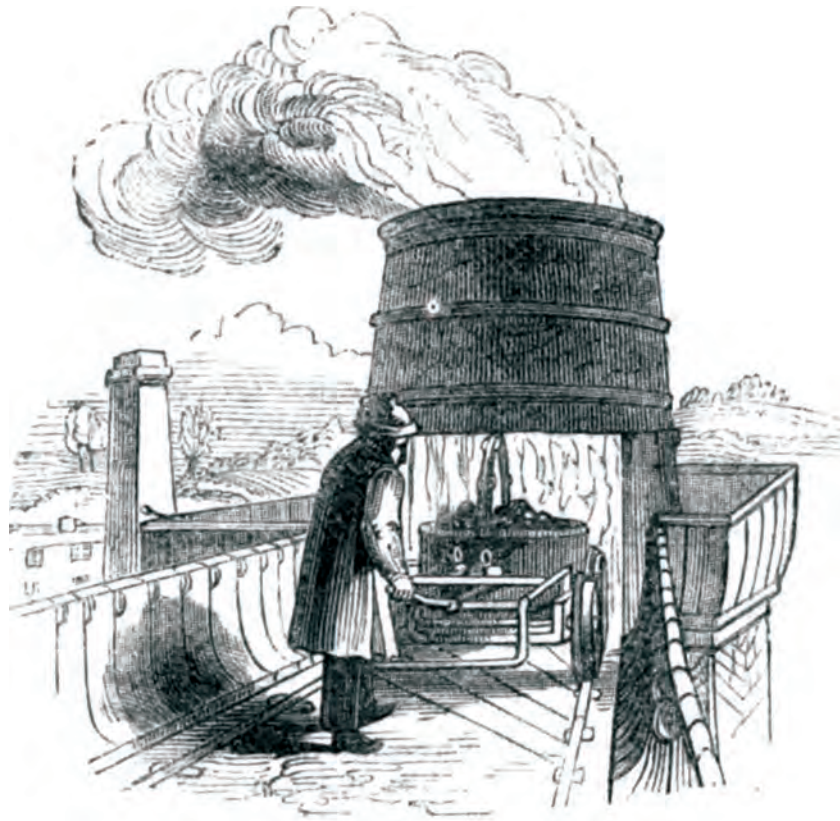
Figure 19: Engraving showing the feeding the furnace at the Butterley ironworks (after Knight 1844), copyright expired
