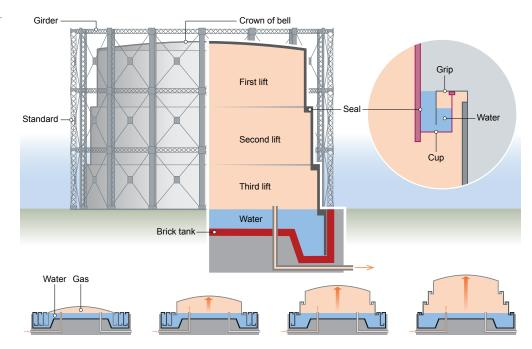
Figure 5: Diagram of a water-sealed gasholder showing the various components including the standards (uprights) and girders of the guide frame, the telescopic bell and the water tank. © Historic England
