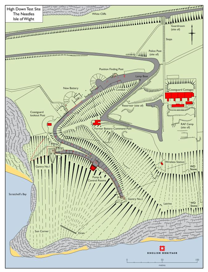
Figure 9 Plan of the High Down Test Facility (c) English Heritage
