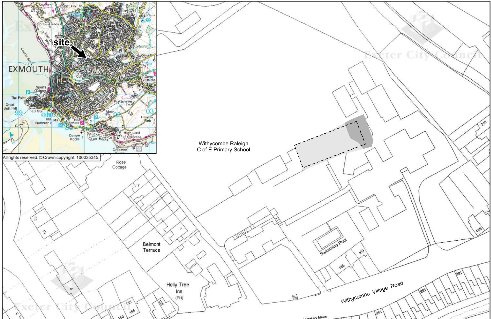
Location of site showing footprint of new building (dashed), area of excavation (light shade) and extent of demolition material (dark shade).
