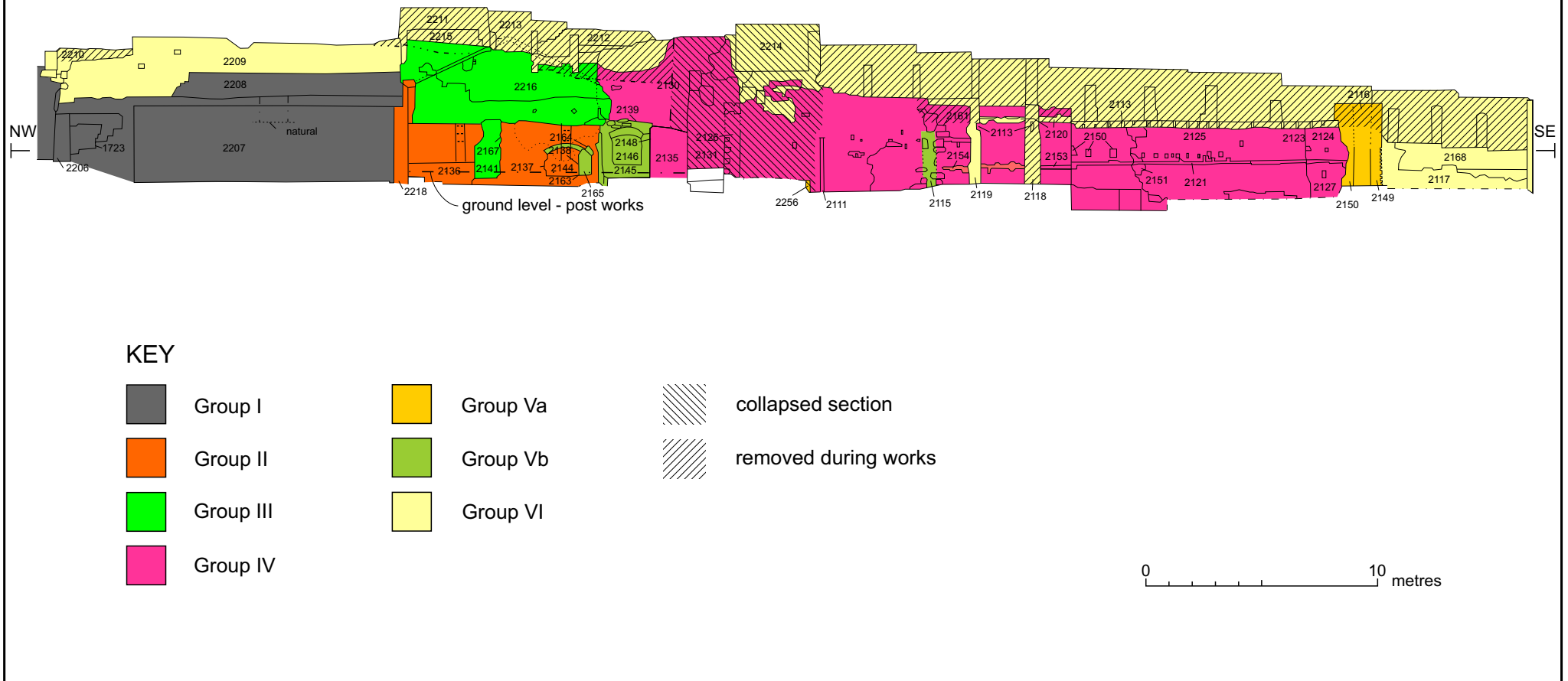
Fig. 3 Phased elevation of the retaining wall, based on drawings prepared in 1989 and 2007.
