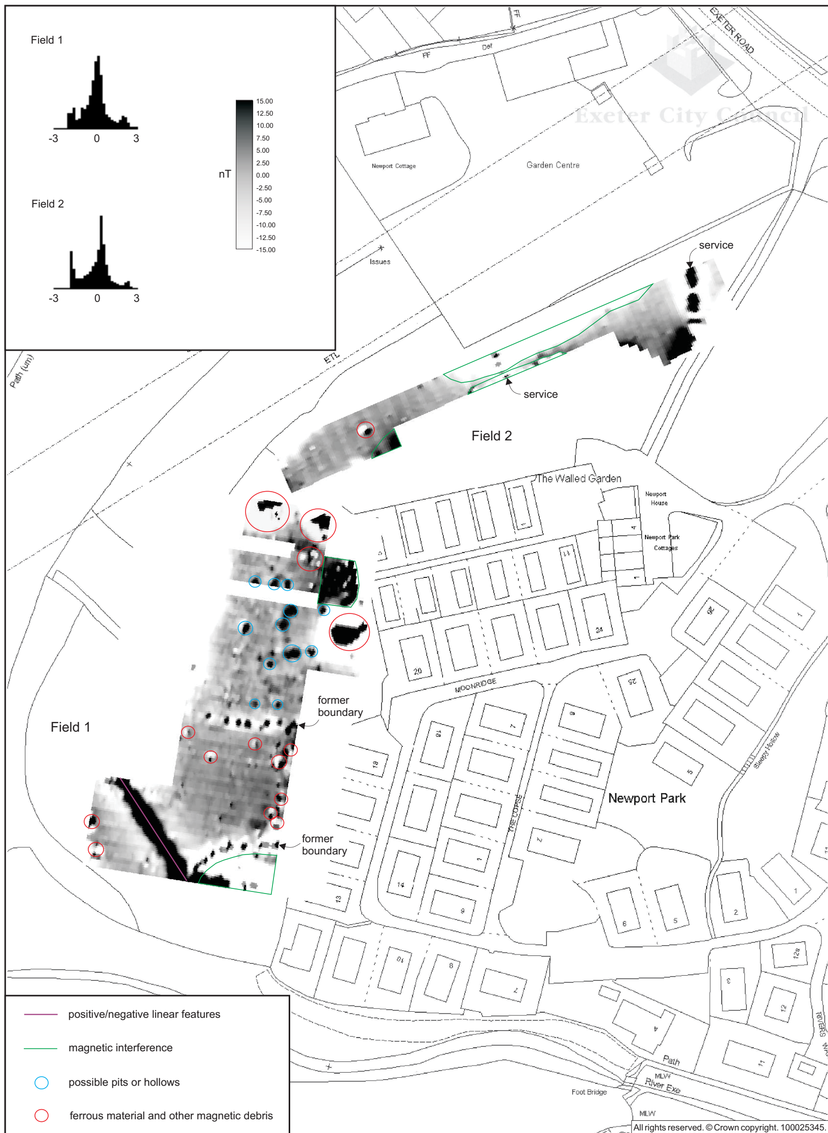
Fig. 4 Interpretation of gradiometer survey results. Scale 1:1000 @ A3.
