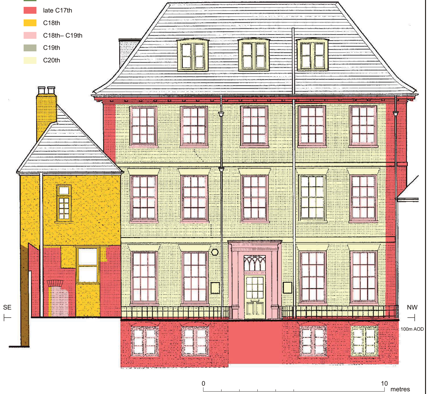
Fig. 32 Phased north-eastern elevation of the north-east range. (Based on a survey by RJD).
