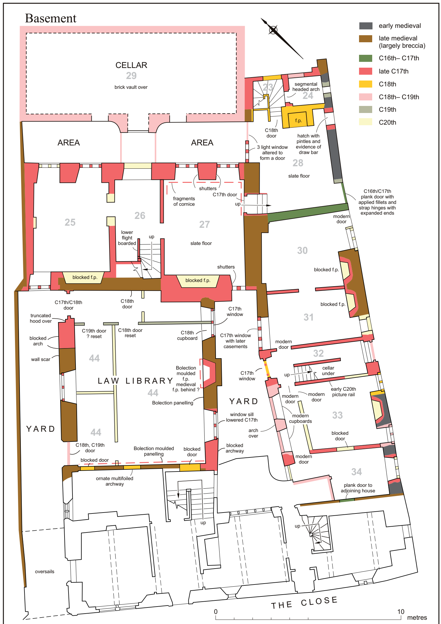
Fig. 24 Phased plan of basement of Notaries House, with ground floor of Law Library and No. 9A. The ground floor of No. 9 is shown in outline. (Based in part on a survey by RJD).
