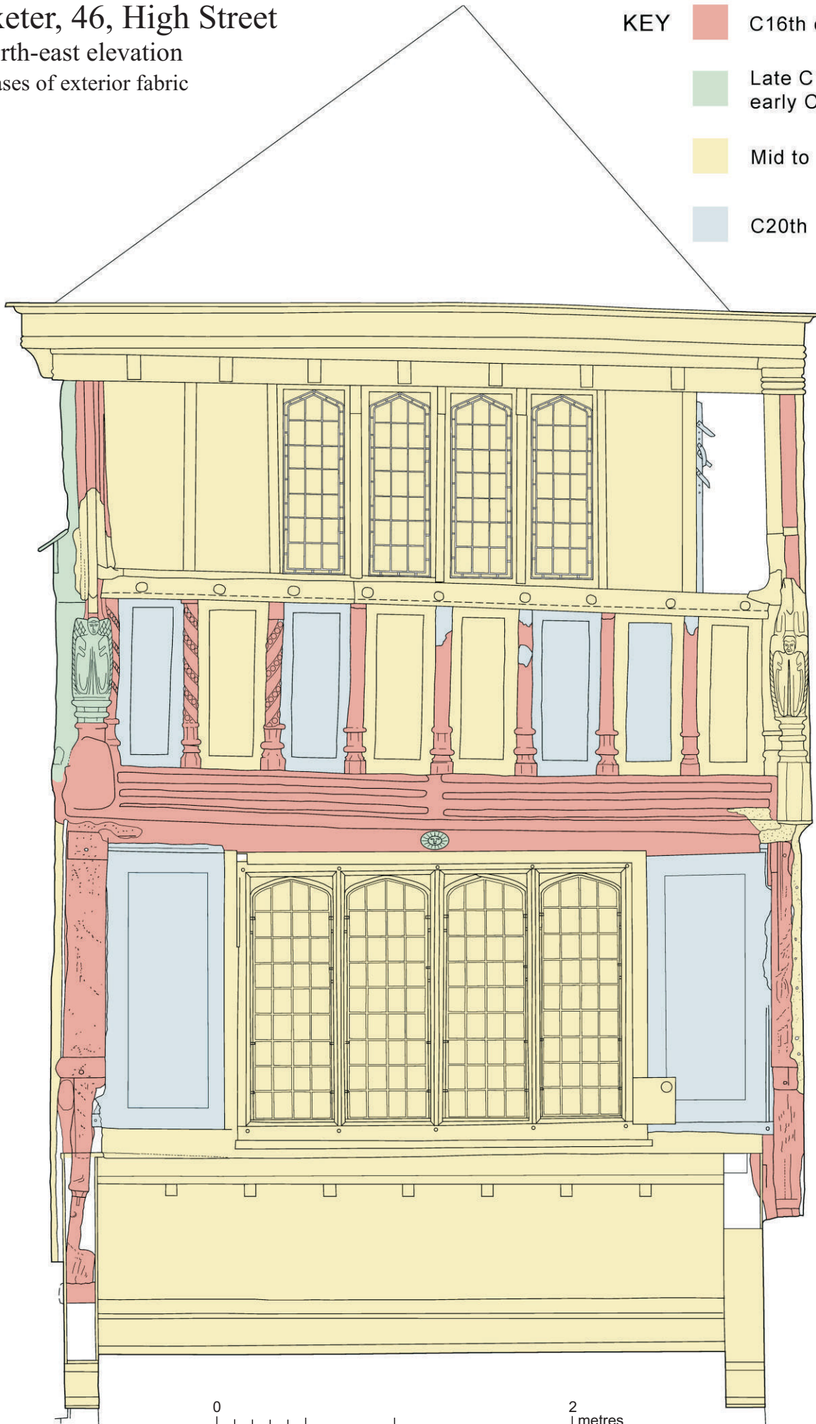
Fig. 14 Phased elevation drawing of the frontage showing the exterior surface fabric prior to works. Scale 1:30.
