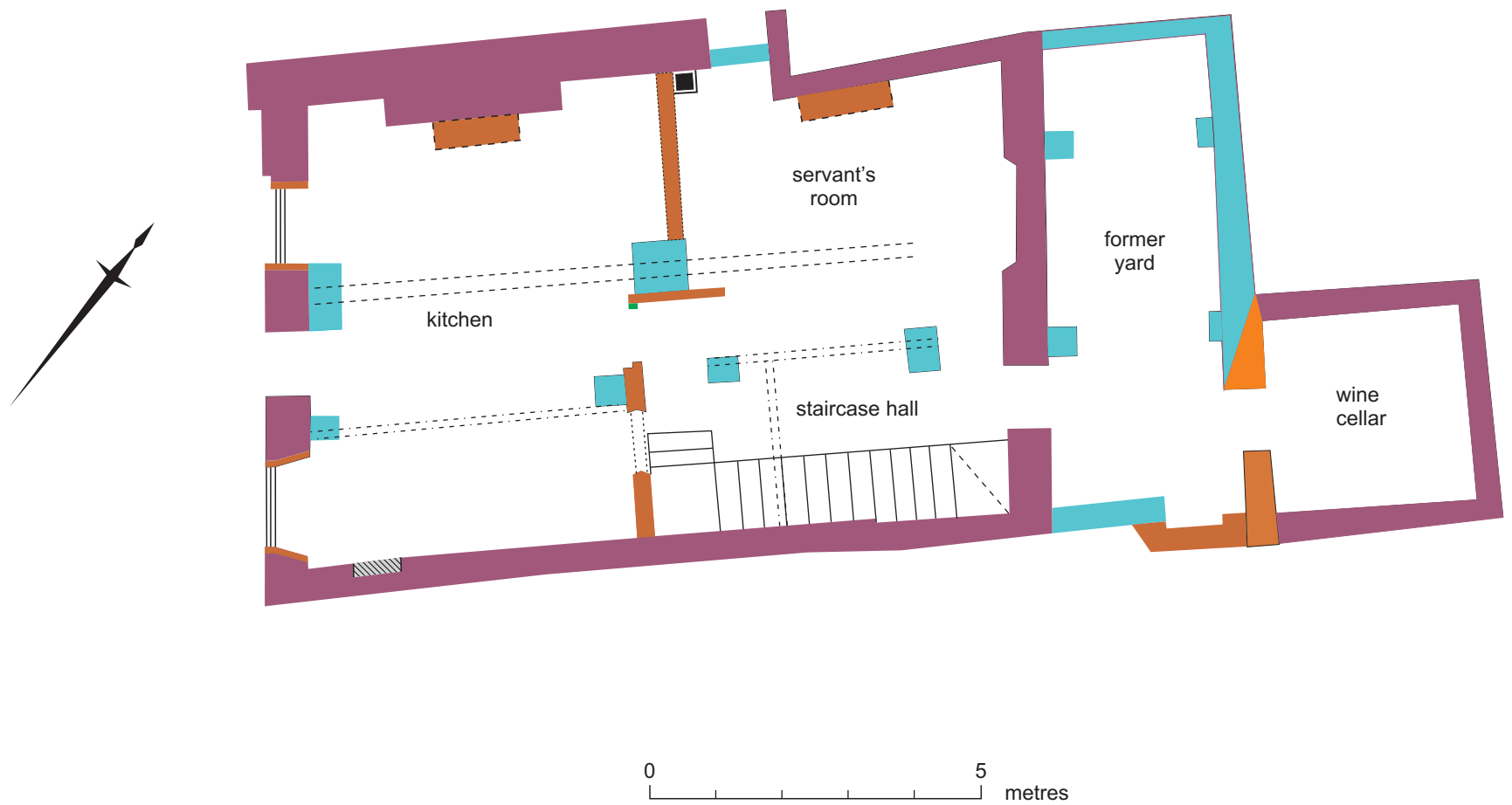
Fig. 2 Plan of the basement showing the existing fabric and suggested room layout. Scale 1:100.
